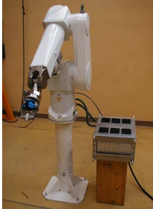
Figure 2-18. RX90 robot fitted with DELTA RAD F/T sensor. Retrieved on 11/09/2014 from [63].
