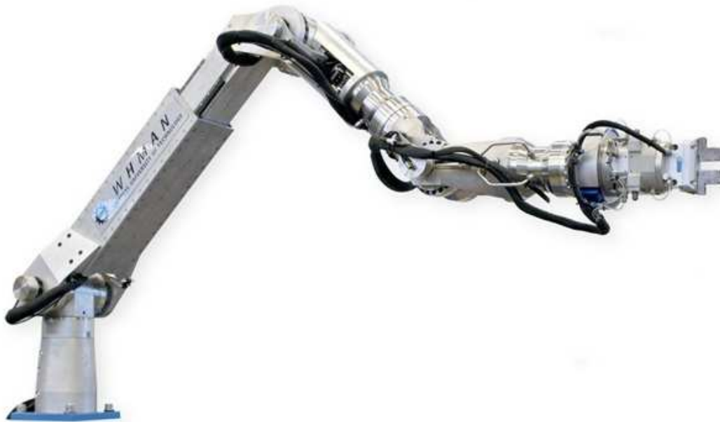
Figure 2-11. WHMAN water based hydraulic manipulator. Retrieved on 7/09/2014 from http://sine.ni.com/cs/app/doc/p/id/cs-14767
