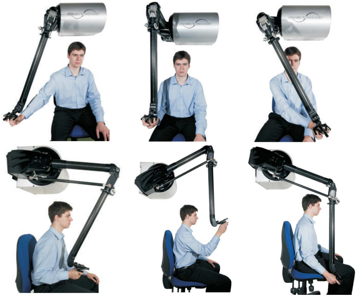
Figure 2-4. Work envelope of Dexter 20, developed by Oxford Technologies Ltd.
