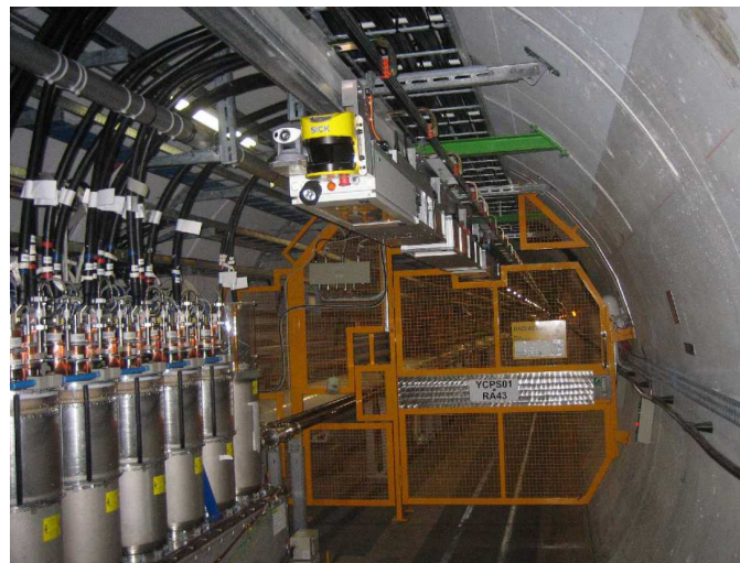
Figure 2-9. TIM monorail inspection train for surveys at LHC.
