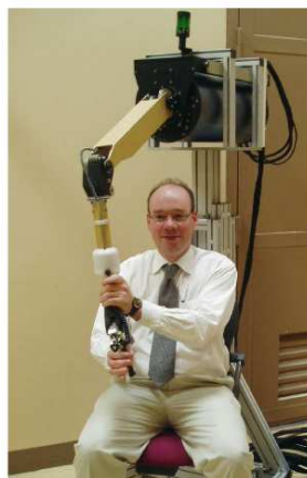
Figure 2-5. Virtuose 6D40-40 master arm designed for manipulation in hostile environments. Retrieved from http://www.est-kl.com on 30/08/14.
