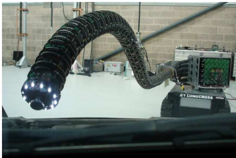
Figure 2-13. OZ robotics snake-arm for survey operations. Retrieved on 10/09/2014 from http://www.ocrobotics.com/products--services/
