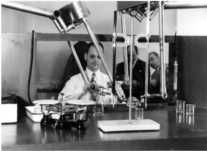
Figure 2-1. Ray Goertz experimenting with mechanically linked manipulators. Retrieved from http://mabe.utk.edu on 28/08/14
