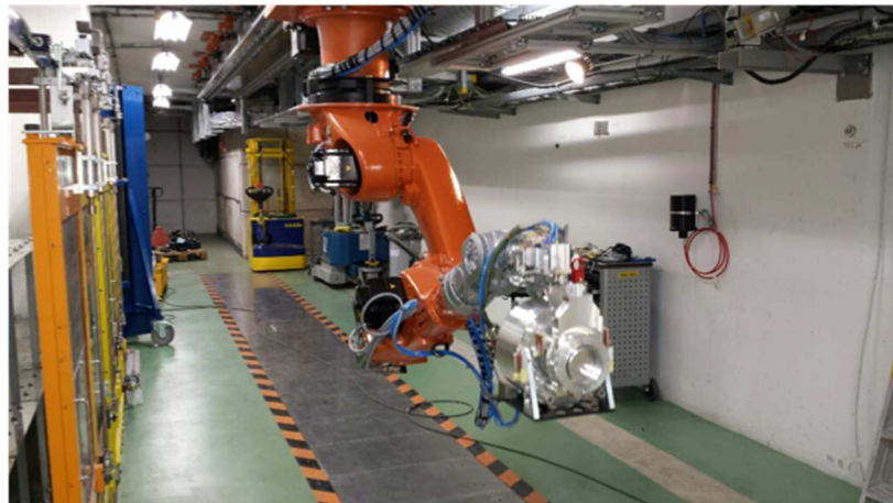
Figure 2-8. KUKA robot transporting an activated target mock-up at ISOLDE facility at CERN. Retrieved from http://home.web.cern.ch/about/updates/2014/08/isolde-back-target-after-shutdown on 30-8-2014.
