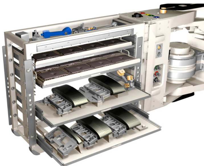
Figure 2-7. Multi drawer task module to be transported by the short articulated boom. Retrieved 23 August 2014, from http://www.ccf.ac.uk/rh.aspx
